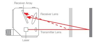
Triangulation sensors determine range by the position of the received light on the receiver array.
