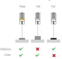
Inspections use distance to verify parts presence and position, and intensity to verify correct color or part orientation
